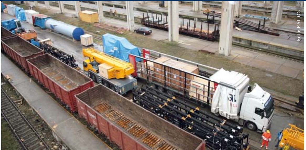
Transshipment of the parts of an industrial furnace complex to broad gauge freight cars at the harbour of Sassnitz-Mukran
