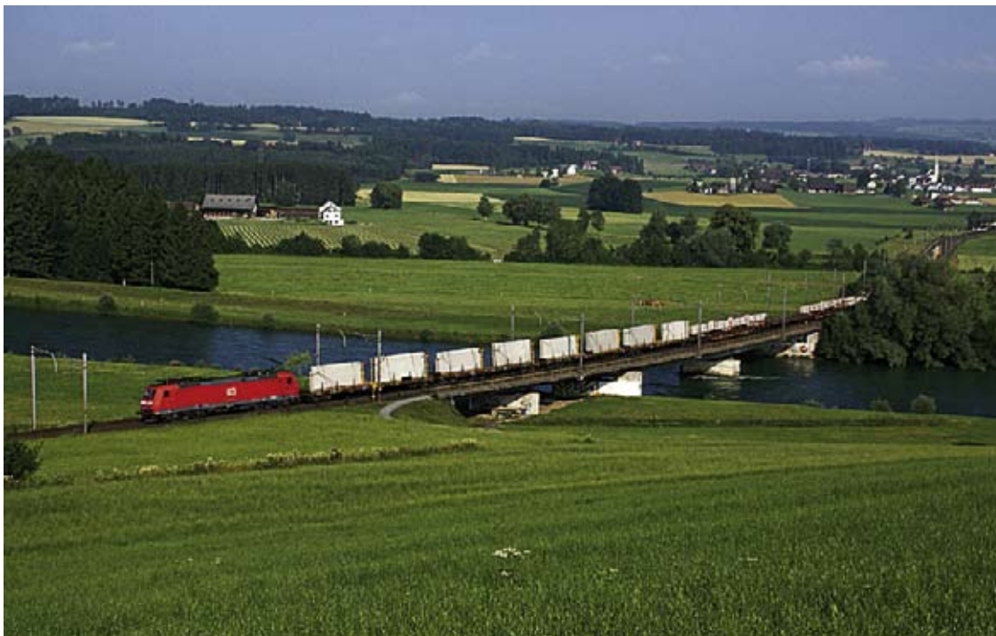
Tubbings on rail: these concrete parts will form the inner lining of the Scheldt tunnel.
