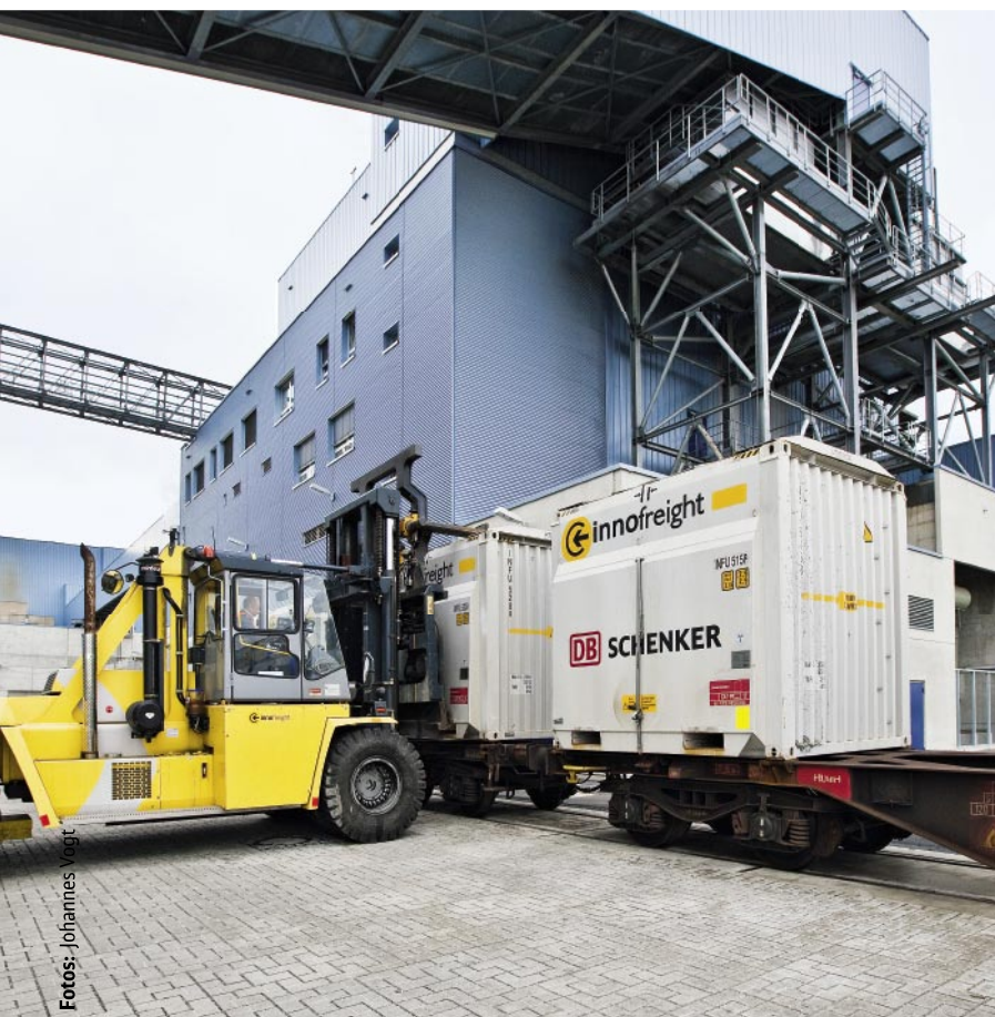
Unloading at the power station. RFID chips clearly identify the individual containers and their contents. A WLAN system tells the forklift driver which dischargepoint to head for.
